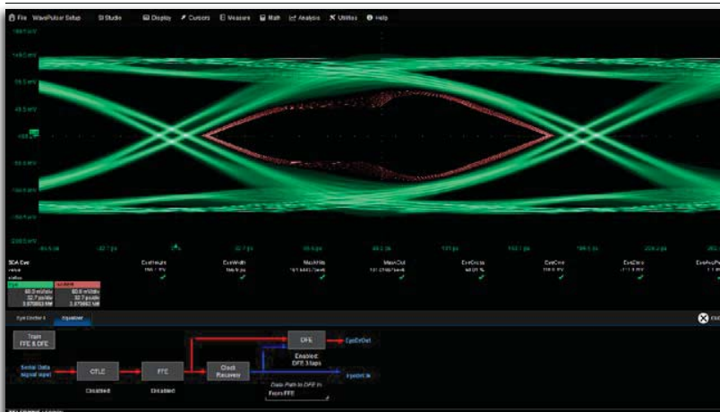
WavePulser 40iX emulates the eye diagrams of the complete serial-data channel.
